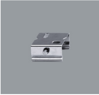
79503.000 Fixing clip Spring steel, galvanised. Load: 20kg. L 33mm. H 14mm.
