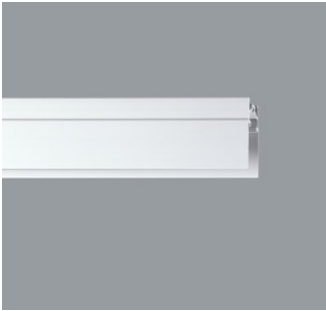
78350.000 Plaster trim profile Aluminium profile, silver anodised. For flush mounting of track in plasterboard ceilings. B 40mm, H 52mm, L 3000mm. Weight 3.00kg
