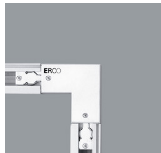
79307.000 3-circuit L-connector Polymer. Earth conductor outside. Feed-in possible. Through-wiring. White 🔌 ⚡ CE
