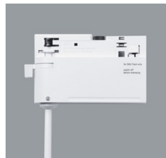
79047.000 ERCO DALI adapter for 250V, 1A pendant luminaire, with strain relief. Polymer. Connection cable 5x0,75mm 2 , L 1500mm. Requirements placed on DALI control gear: DALI input suitable for mains voltage, max. capacity 750pF. Not suitable for DALI singlet. White Weight 0.39kg CE
