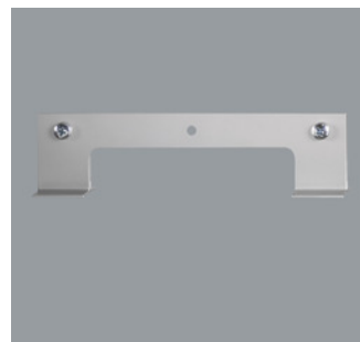
79501.000 Suspension bridge for direct track coupler connection. Metal, galvanised. Subsequent mounting of suspension bridge in ERCO track possible. Load: 20kg. L 180mm, H 47mm.
