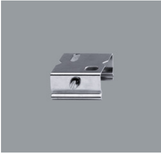
79503.000 Fixing clip Spring steel, galvanised. Load: 20kg. L 33mm. 14mm.
